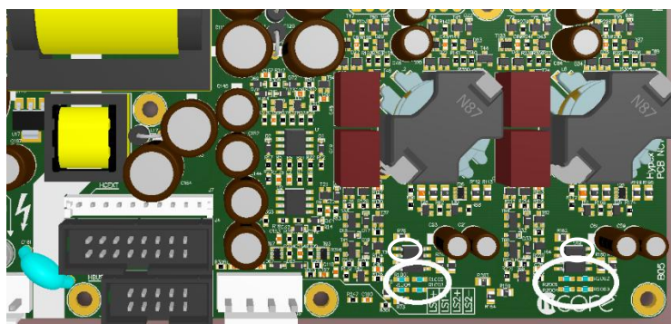
Figure 1 Placement of the bypass resistors
