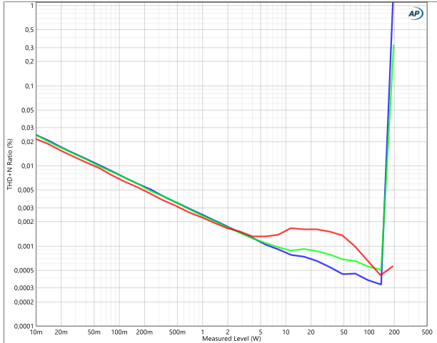
THD+N vs. power at 100Hz (blue), 1kHz (green) and 6kHz (red) (2Ω).
