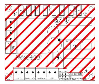
This symbol indicates the presence of hazardous voltages at accessible conductive terminals on the board.
